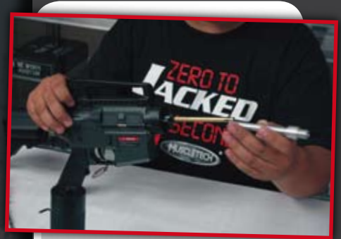
Insert the aluminum outer barrel
