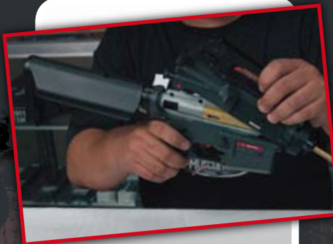
Close the receiver assembly
