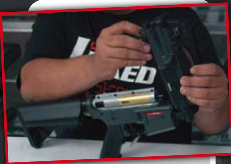
Re-insert the inner barrel into the receiver
