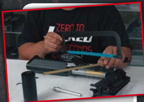
A hack saw was used to cut the barrel.
